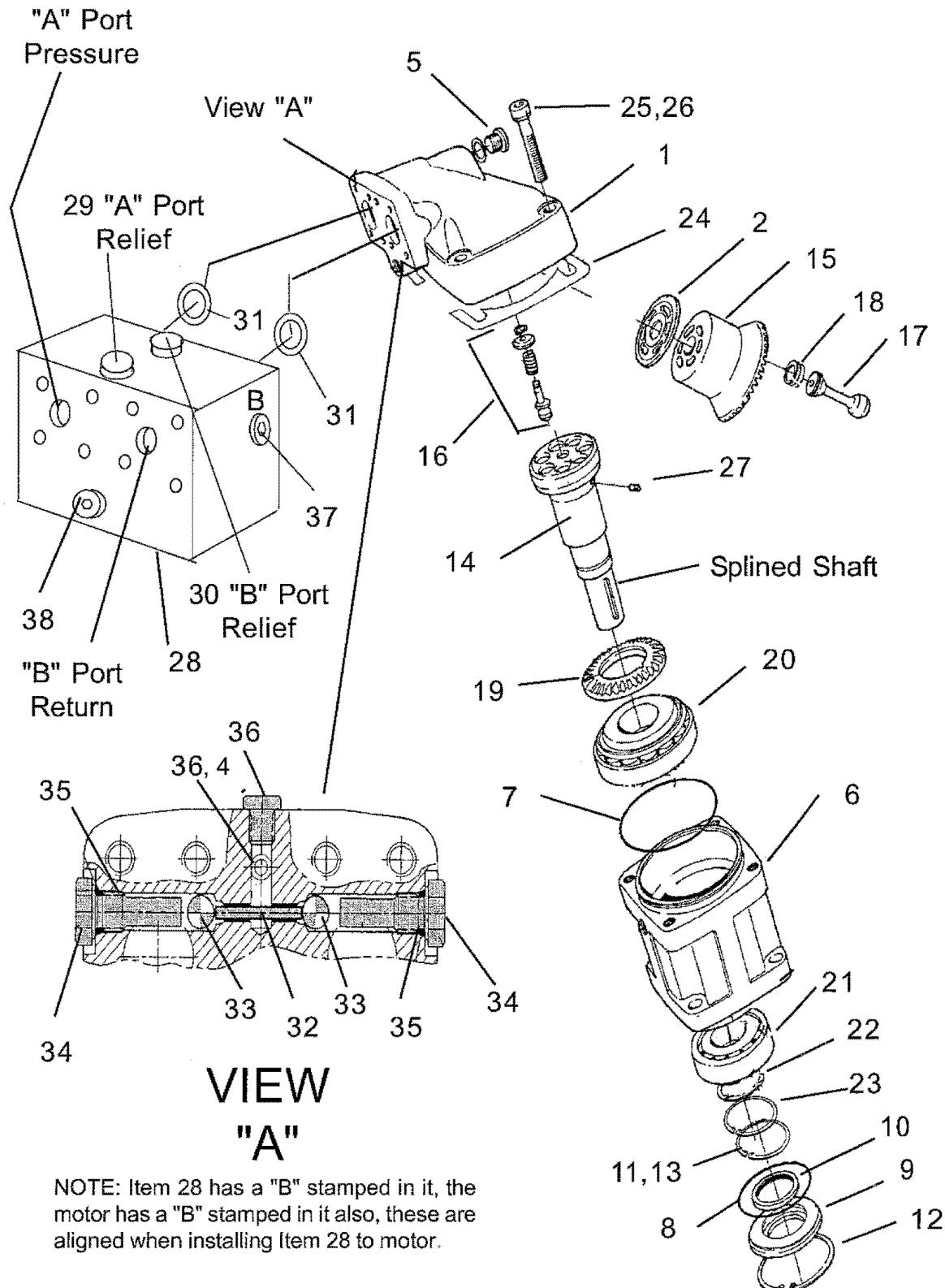
NOTE: Item 28 has a "B" stamped in it, the motor has a "B" stamped in it also, these are aligned when installing Item 28 to motor.
